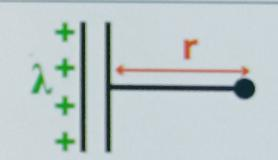
Electric Field Near an Infinite Plane Sheet of Charge
